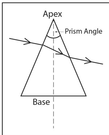
Again, the two “plane” prism surfaces meet at the apex, creating the prism angle, the opposite of which is the base. Prism is always written referencing the direction of its base. The deviating properties of a prism are directly proportional to its prism angle: as the angle increases, as does the degree of deviation. As stated previously, by definition, a 1D prism will displace an image 1cm at a distance of 1 meter.
