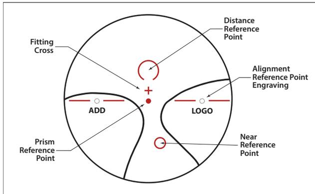
In a PAL, ground prism can only be accurately verified through the Prism Reference Point (PRP) – the point below the fitting cross, 17mm from each engraved circle. This actually makes verifying prism in a PAL much easier than other lens designs – it’s definitive!
