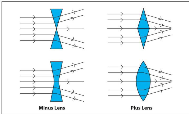
A plus lens is basically 2 prisms arranged base to base, and a minus lens is basically 2 prisms arranged apex to apex. If you move a plus lens in front of your eye, you will see “against motion”. Do the same with a minus lens, you’ll see “with motion.” The rules mentioned above explain this prismatic deviation and why lenses function the way they do.
